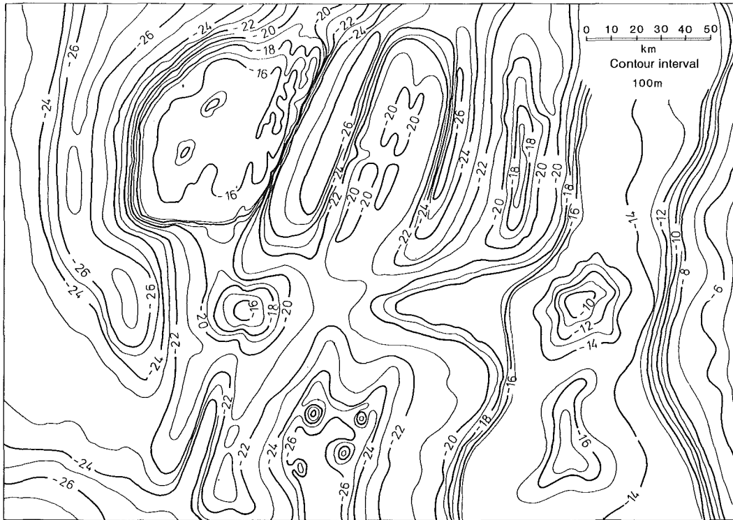
Fig. 9 Structural form elements shown as depths down to an unconformity surface (seismic reflector) on an idealized subsurface map of a continental shelf. The form elements are identified and given unit designations in figure 10.
